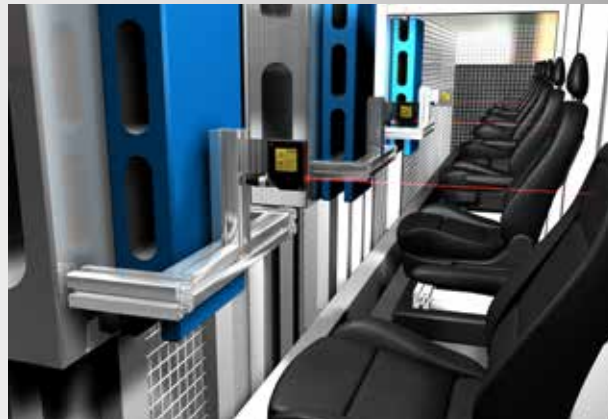
Quality inspection of seats The functional inspection of the seats is carried out using automated, mechanical adjustment of the seat and a downstream measurement of the positions using the OADM 20 sensors.
