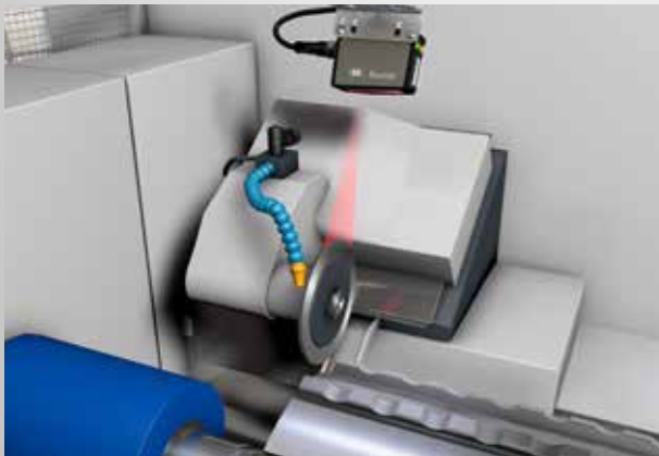
Measurement of the diameter of a grinding disk Thanks to the automatic calculation of the average, OM70 multi-spot sensors allow the optimum positioning of very rough grinding wheels in relation to a workpiece.
