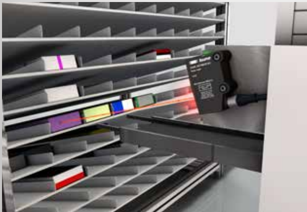
Checking the filling of a high-bay storage system By means of measurements even over distances of up to 1000 mm, the OADK 25 controls automatic filling systems in the logistics sector, thus reducing handling and material costs.
