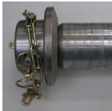
Figure 4-6 Securing the lifting rods
