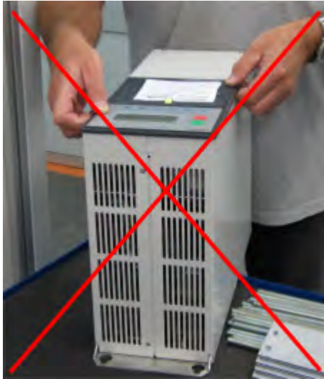
Lifting compact devices - wrong
