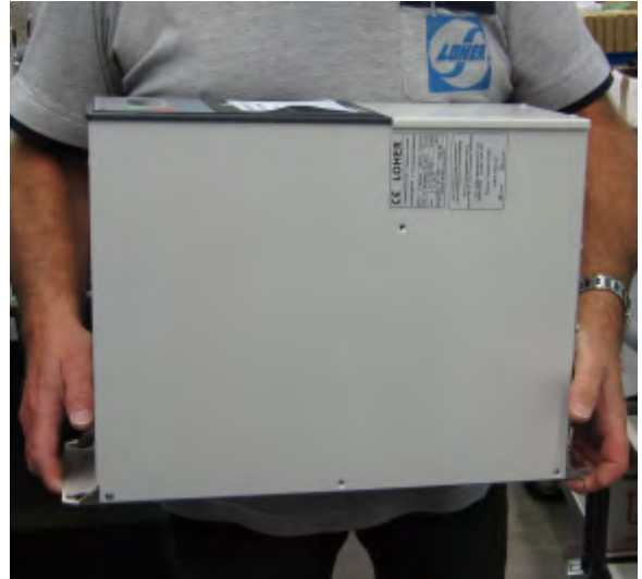
Lifting compact devices - correct
