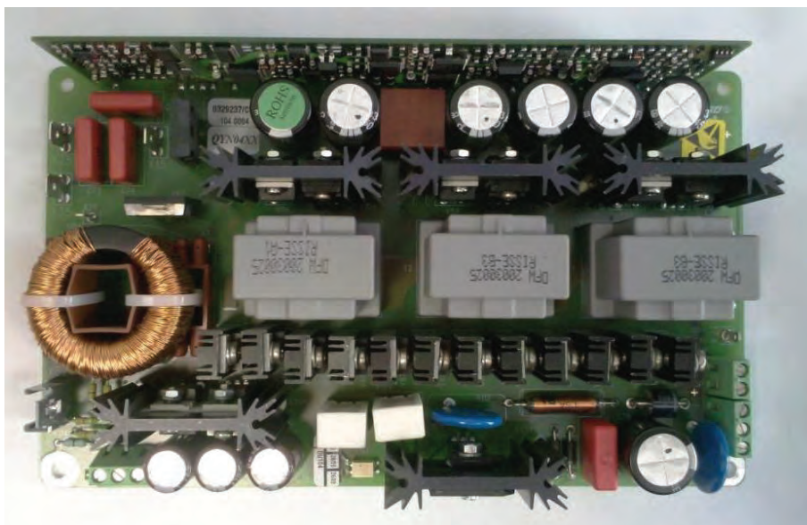
Figure 3-9 PC board of the pre-switch mode power supply (pre SMPS 300W)
