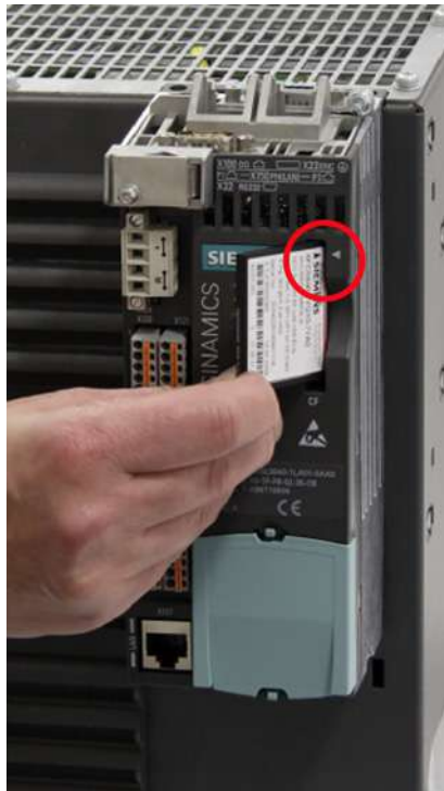
Figure 7-5 CU310-2 PN Inserting the memory card
