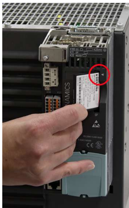
Figure 7-12 CU310-2 DP Inserting the memory card
