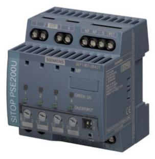
SITOP PSE200U SELECTIVITY MODULE 3A SITOP PSE200U 3 A Selectivity module 4-channel input: DC 24 V/12 A output: 24 V DC/4x 3 A Level adjustable 0.5-3 A mit status message for each output
