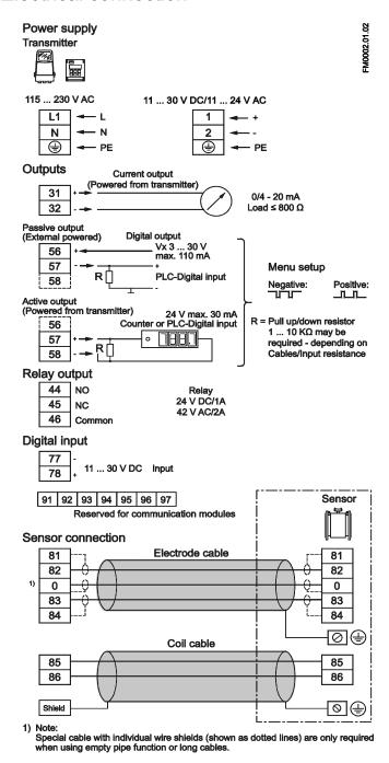
Figure 5-1 Wiring diagram
