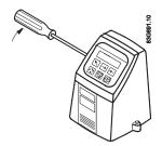
2. Loosen the four screws retaining keypad.
