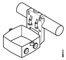
Figure 4-8 Pipe mounting - horizontal
