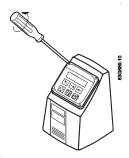
3. Withdraw keypad and turn it to required orientation.
