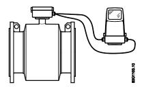
Figure 4-2 Remote installation
