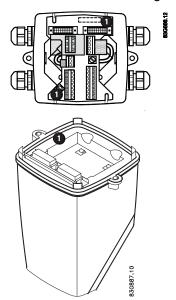
2. Drill through marked drilling holes in terminal box and transmitter/lid. Seal transmitter externally as shown below.
