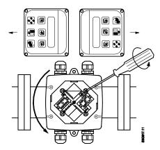
Figure 4-10 Terminal box can be rotated ±90° in order to optimize viewing angle of transmitter display/keypad
