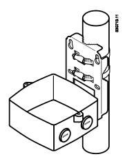
Figure 4-7 Pipe mounting - vertical
