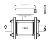
Potential equalization with electrically conductive graphite gaskets
