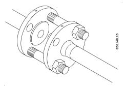
Figure 4-6 First place three stay-bolts to locate the sensor
