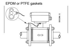
Potential equalization using earth strap supplied
