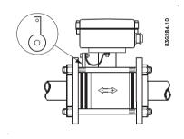
Potential equalization using separate potential equalization ring
