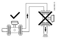
Figure 4-3 Correct installation at low point before outlet
