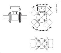
Figure 4-5 Horizontal installation, various terminal box positions
