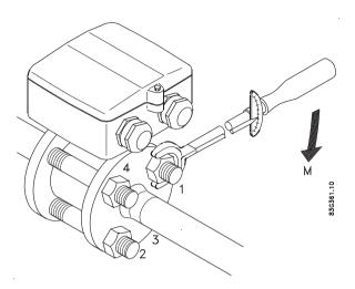
The bolts must be tightened using up to 50% of the max. tightening torque for the pipe dimensions stated. The max. tightening torque for different size pipes is given in the table.
