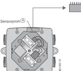
4. Fit the ½" NPT or M20 cable glands for supply and output cables.
