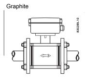
Potential equalization with electrically graphite gaskets
