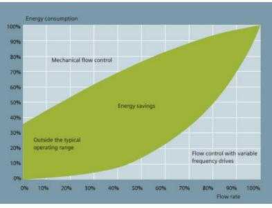
Especially energy saving for pump, fan and compressor applications
