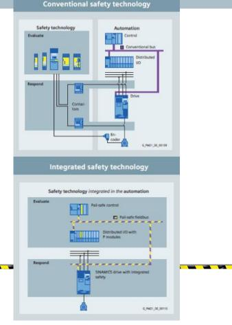
Integrated safety technology reduces the umber components and wiring costs
